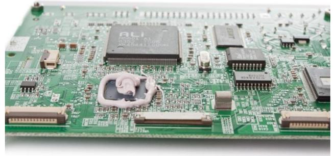
Photo 2, 3: shows thermal conductive parker paste (TIM) placed on the soldered DUT and the surrounding components
