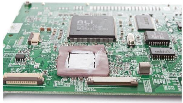
**Photo 5** shows device plunger contacting the entire area of the soldered device and the frame shaped thermal pad.
